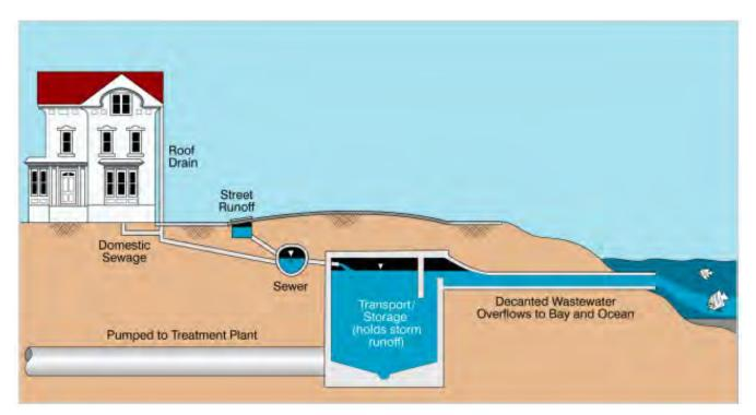
Figure 96. Typical features of San Francisco's Combined Sewer System (SFPUC, 2018c).
