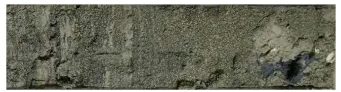
Figure 86. Fill sample from 9.1 to 9.4 m (30 to 31 ft) showing poorly graded sand with sharply defined clay and silt laminations (ENGEO, 2015).
