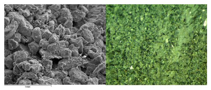
Figure 89. Left: SEM image of tightly packed sand with abundant fines and clay cement; Right: photomicrograph of shoal sand with thin clay lenses (ENGEO, 2015).
