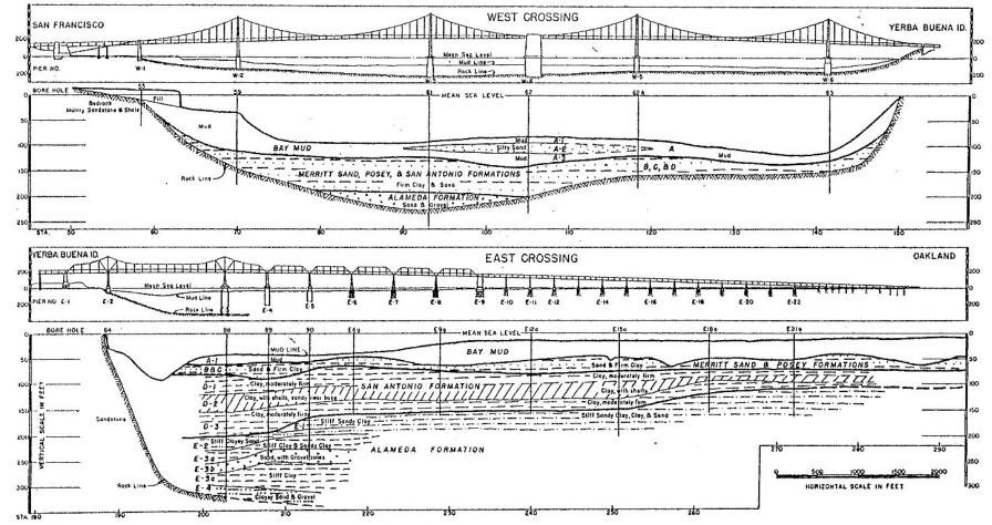
FIGURE 4.—PROFILE OF SEDIMENTS, PARALLEL CROSSING, SAN FRANCISCO BAY
