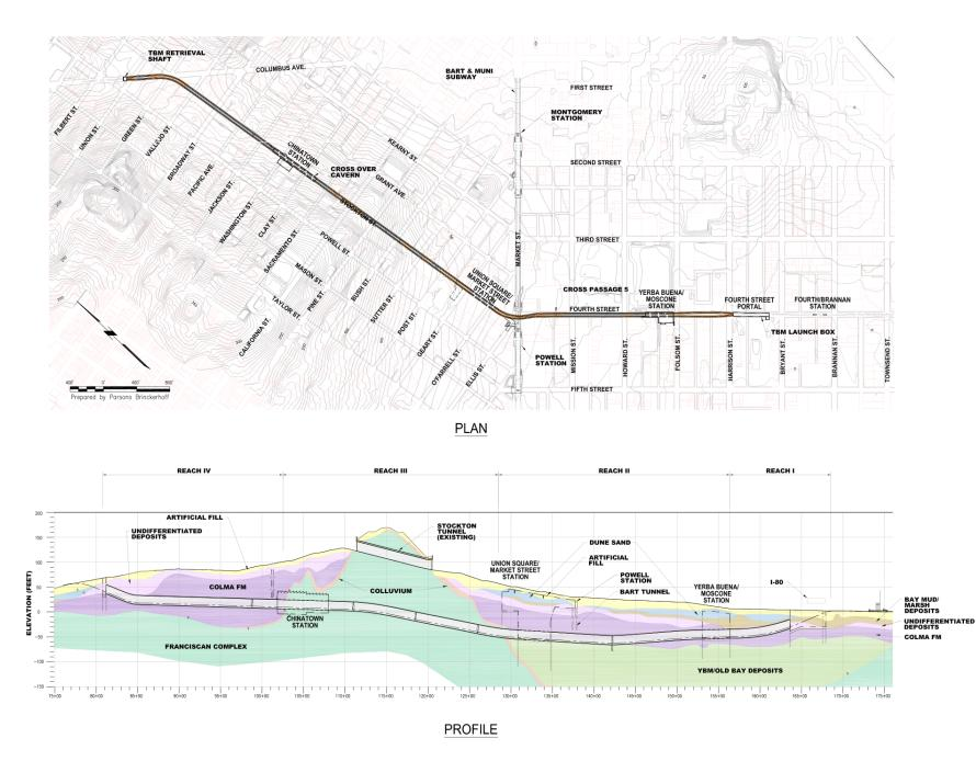
Figure 94. Plan and Profile for the Phase 2 of the Central Subway project. Dk green—Franciscan bedrock; orange—Colluvium; Lt green—YBM/Old Bay deposits; purple—Colma Fm; Lt purple—Undiff. deposits; Ochre—Young Bay Mud; blue—dune sand; Yellow—fill. (Figure from WSP USA, 2018).
