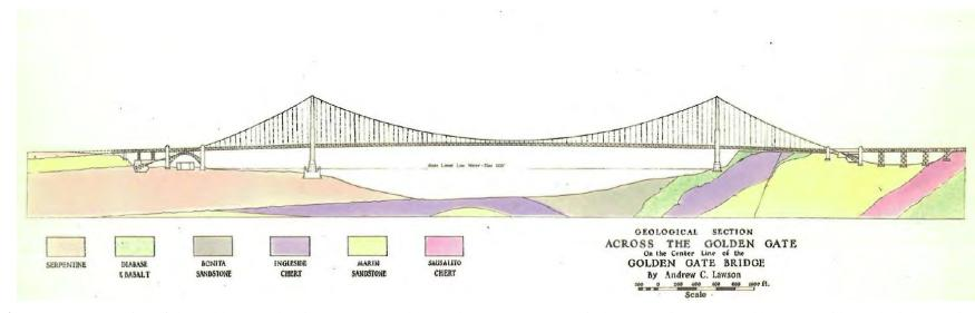
Figure 75. Cross section of the Golden Gate looking west prepared by Andrew Lawson, no vertical exaggeration. From Golden Gate Bridge and Highway District, Investigation of criticism of foundation by Bailey Willis, November 27, 1934.
