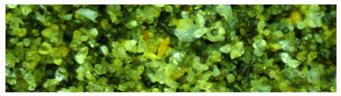
Figure 87. Photomicrograph of clean sand at 9.6 m (31.5 ft) (grain size predominantly 0.4 mm to 0.1 mm) (ENGEO, 2015).
