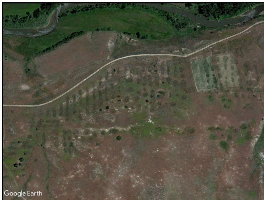
Figure 3-19 June 25 th 2017 satellite image of room and pillar mine subsidence near Sheridan, Wyoming, above the Old Monarch Mine in operation from 1904 to 1921. Overburden thickness is estimated to be 10 to 15 meters. Circular pits and depressions are from roof collapse between pillars. Smaller holes are caused by piping failure as surface water drains into tensional cracks. Image taken from Google Earth.
