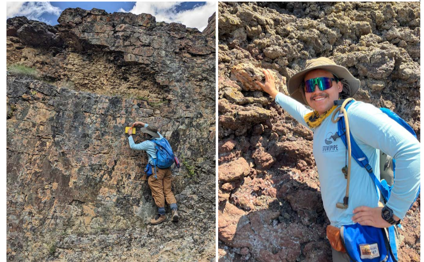
[LEFT] Taking the strike, dip, trend, and plunge measurements of a prominent fault surface in Banana Canyon within the Challis region of SE Idaho. [RIGHT] Getting familiar with the basaltic features at Craters of the Moon near Arco, Idaho.
