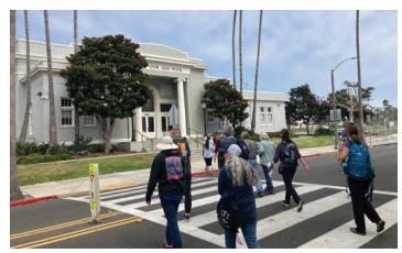
FIGURE 5, STOP #5. APPROACHING THE DWYER SCHOOL GYMNASIUM, ONE OF THE FEW STRUCTURES THAT SURVIVED THE 1933 M6.4 LONG BEACH EARTHQUAKE BECAUSE IT USED REINFORCED CONCRETE INSTEAD OF THE MASONRY CONSTRUCTION TYPICAL OF THE TIME.
