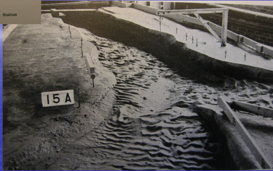
Natural sand bed channel (lower left); dredged channel (upper right); and impact of structural dikes (lower right)
