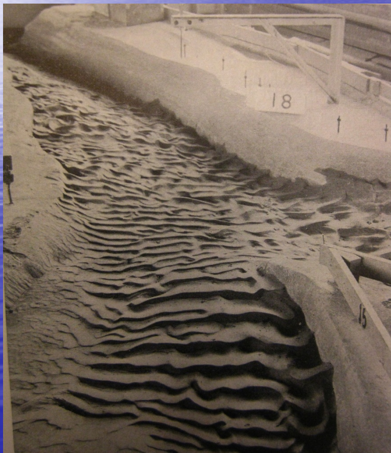
Natural sand bed channel (lower left); dredged channel (upper right); and impact of structural dikes (lower right)
